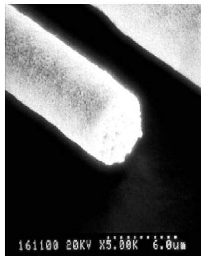
Fig. 5 SEM photograph of a PT fiber cross section which was not subjected to solvothermal treatment.
